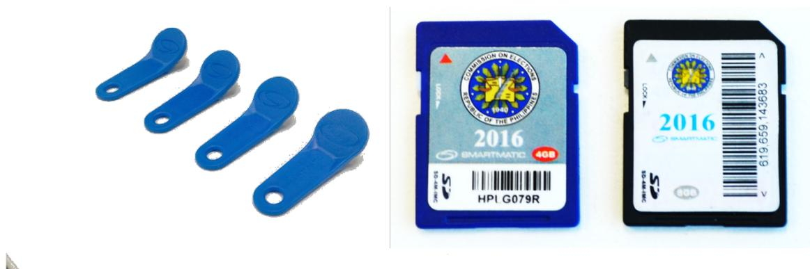
Figure 1. Official iButtons and SD Cards used in 2016 NLE (Blue SD Card is WORM)
