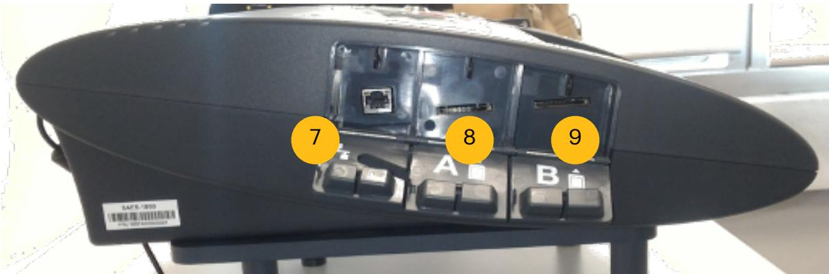
Figure B. Side view of the SAES 1800plus showing SD card slots
