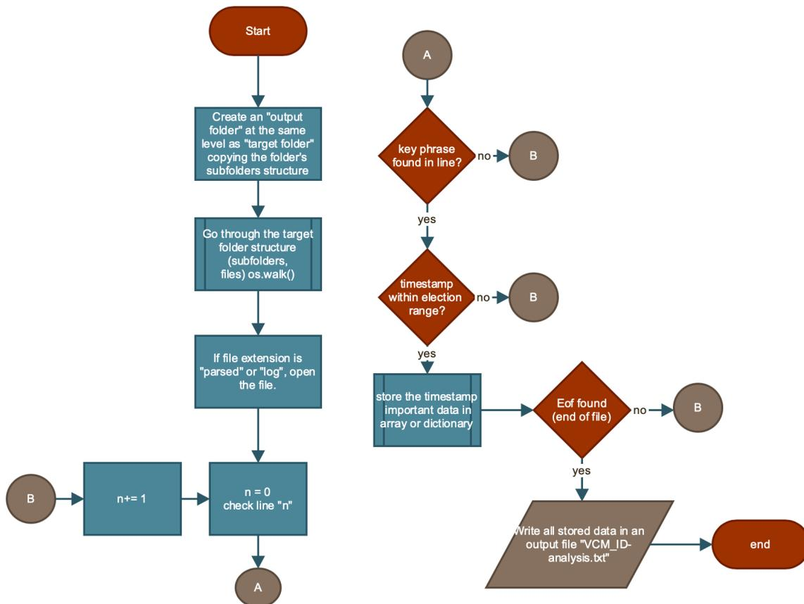
Figure 8. Program Flow Logic for analyzing the VCM audit log files
