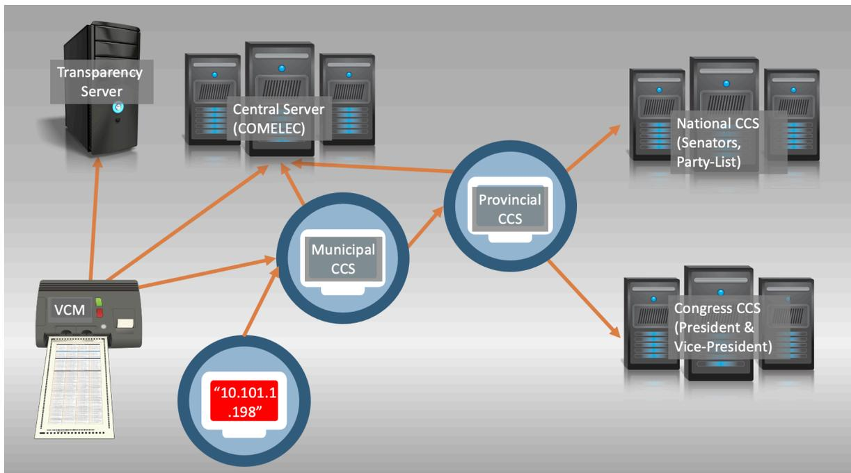
Figure 12. Modified Transmission Flow due to “10.101.1.198”
